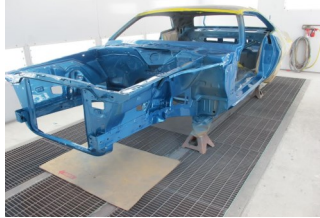
Edged and start prepping for final paint.
