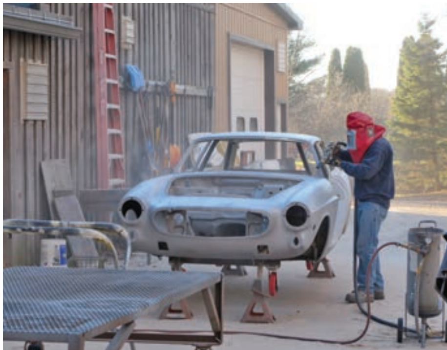
The 1800 was completely disassembled, with all parts meticulously cataloged, before being sandblasted and then primed in epoxy.
