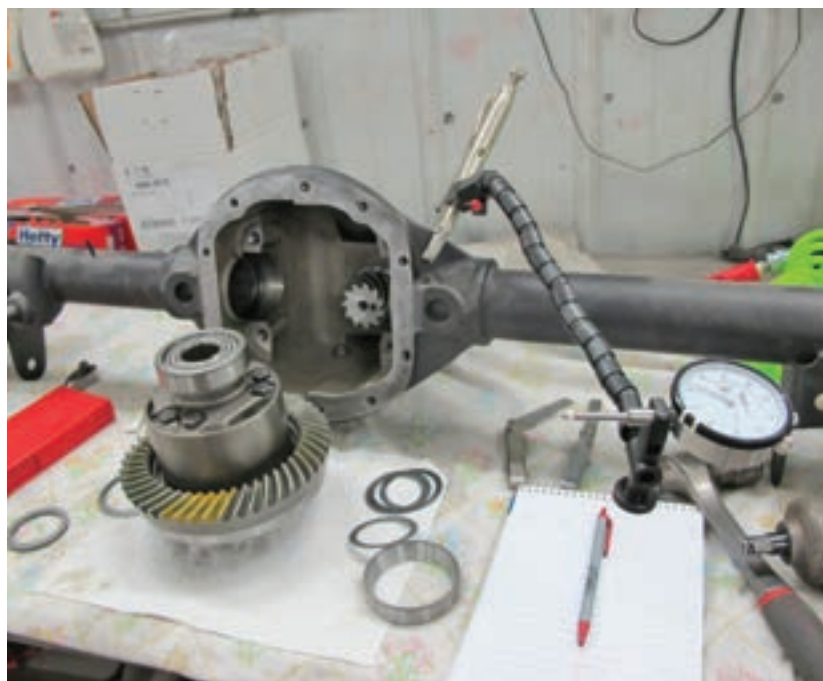
The rear axle was also disassembled, sandblasted, and painted. It was then reassembled with a new ring and pinion setup (4.27:1), new bearings, and a Trutrac limited slip unit.
