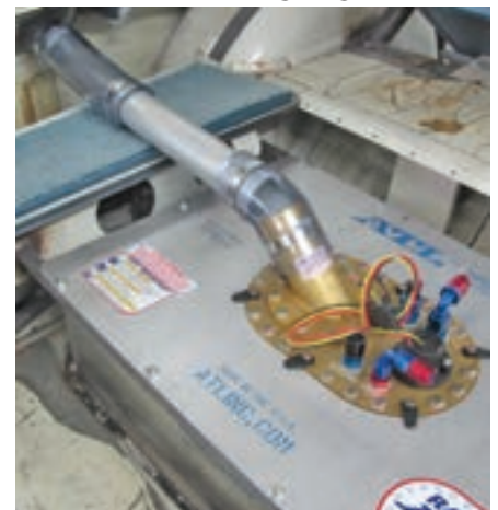
The fuel tank was replaced with an aluminum fuel cell holding 22 gallons.
