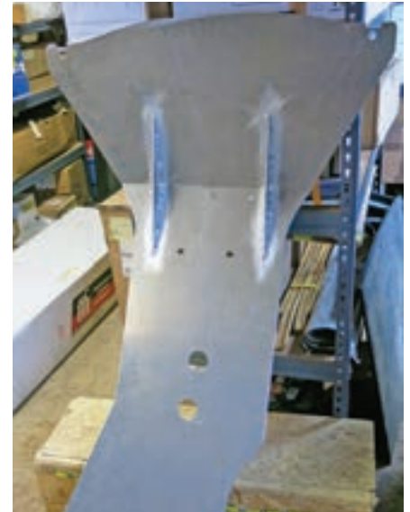
A large aluminum skid plate was fabricated to protect the bottom of the car, including the front cross member, transmission, and drive shaft.
